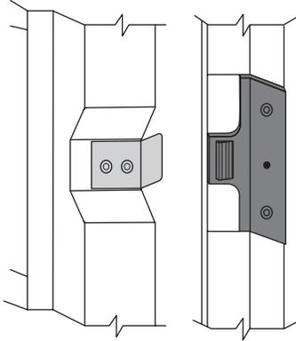
**A1 Installing valve wall:**
