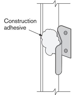
**B2 Installing valve wall:**
