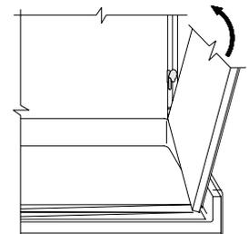
**6** With walls firmly pushed down and front edge of side wall aligned with front edge of pan, screw through side wall flanges into framing.
