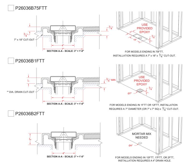
ALL SHOWN AS INSTALLED WITH SOLID BRASS, NO-CAULK DRAIN FITTING (INCLUDED, INSTALLED BY OTHERS)
