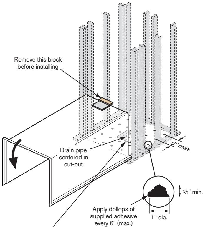
**!** Drain cut-out must be 8" diameter or 8" x 8".
